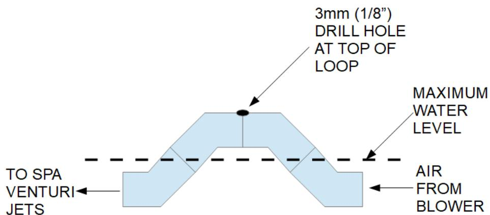
**NOTE:** The top of the loop must be above the maximum water level in the spa.
