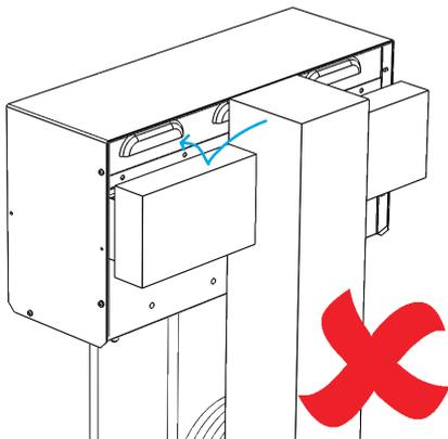
*Without a backing board unacceptable water ingress may occur in severe wind and rain weather conditions. This can damage the unit and void the manufacturers warranty.*
