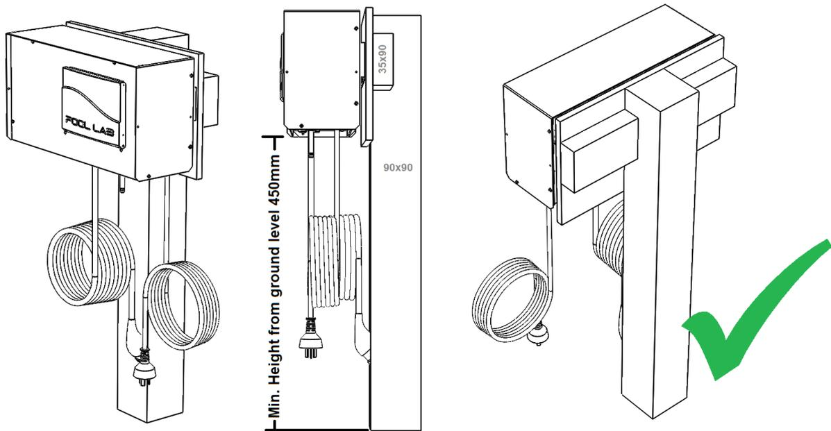
*Example: Mineral Lab Chlorinator mounted to a freestanding post with a backing board. Ensure the post is secure and all materials used are suitably weatherproofed. The bottom of the unit must be mounted a minimum of 450mm from ground level.*
