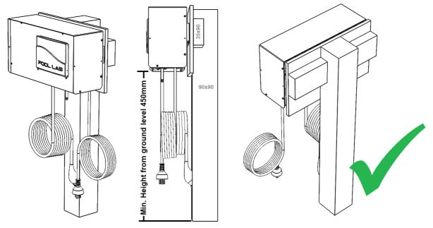
Example: Pool Lab Salt Chlorinator mounted to a freestanding post with a backing board. Ensure the post is secure and all materials used are suitably weatherproofed. The bottom of the unit must be mounted a minimum of 450mm from ground level.
