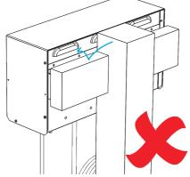
Without a backing board unacceptable water ingress may occur in severe wind and rain weather conditions. This can damage the unit and void the manufacturers warranty.
