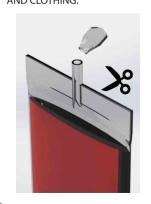
**6.** PUSH CONNECTOR INTO OPEN TUBE
