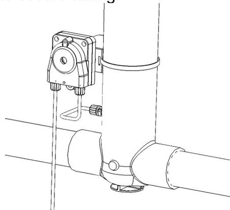
**Step 5.** Insert loose end of 5mm tubing into Fume Stop Cap as shown. Ensure tubing can reach bottom of reservoir, and cut to length if required. Fit tubing weight to bottom end of tube.
