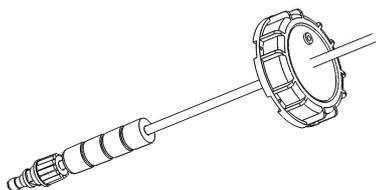
**Step 6.** Fit Fume Stop Cap to Acid reservoir, and pass through enough tubing to reach bottom of the drum. Lightly tighten lock nut to secure tube.
