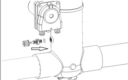
**Step 3.** Install a short length of 5mm tubing to connect the Acid Pump outlet to the Acid Injector. Tighten lock nuts by hand to secure tubing.
