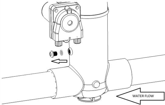
**Step 2.** Install the Acid Injector. Ensure the o-ring is in place, and tighten by hand only.
