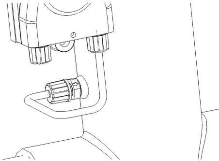
**Step 4.** Install the remaining 5mm tubing to the Acid Pump inlet. Tighten lock nut by hand to secure tubing.
