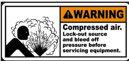
Due to the potential risk that can be involved, it is recommended that the pressure test be kept to the minimum time required by the local code. Do not allow people to work around the system when the circulation system is under the pressure test. Post appropriate warning signs and establish a barrier around the pressurized equipment. If the equipment is located in an equipment room, lock the door and post a warning sign.
