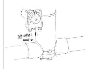
**Step 3.** Install a short length of 5mm tubing to connect the Acid Pump outlet to the Acid Injector. Tighten lock nuts by hand to secure tubing.
