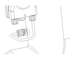
**Step 4.** Install the remaining 5mm tubing to the Acid Pump inlet. Tighten lock nut by hand to secure tubing.
