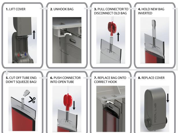
NOTE: After installing new reagent bags, prime the reagent lines by either:
