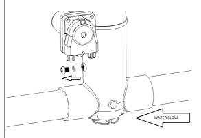
**Step 2.** Install the Acid Injector. Ensure the o-ring is in place, and tighten by hand only.
